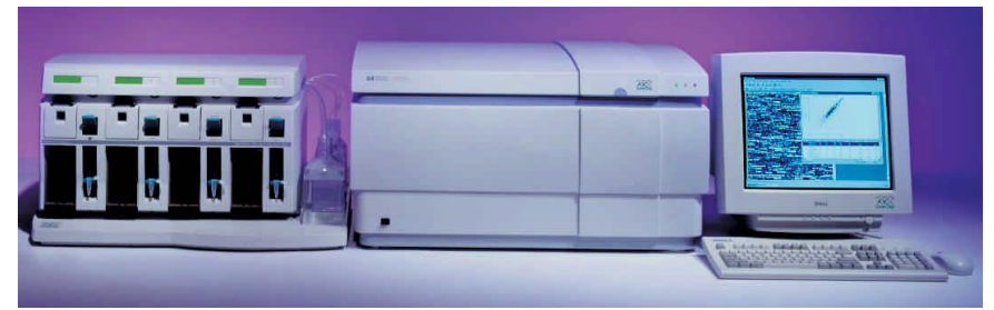
Figure 4. Hardware for the Affymetrix platform. The fluidics station (on the left, for washing and staining) can process up to 4 GeneChips simultaneously in about 90 minutes. The epifluorescence scanner (middle) has a maximum resolution of 3 microns and scans each chip twice over 10 minutes. Both machines are software-controlled.
