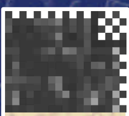
Affymetrix GeneChip snapshot depicting a processed raw image. Each square cell contains the same 25mer probe and is 18 microns across. About half a million such cells are present on each genome-wide expression microarray such as the human U133A and B set. The chequered edge is a spiked control oligo which allows monitoring quality and providing landmarks for a grid overlay.
